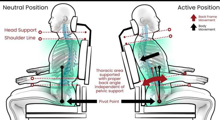
The segmented back support system provides stationary pelvic support and a moving thoracic segment. The system also incorporates an anatomical pivot point, contributing to improved stability. Postural changes can help support functions such as respiration, digestion, peer engagement, fatigue management, and performing routine movements, to name a few. All secondary positioning supports attached to the thoracic segment move in unison with the body, reducing the frequency of repositioning events.
