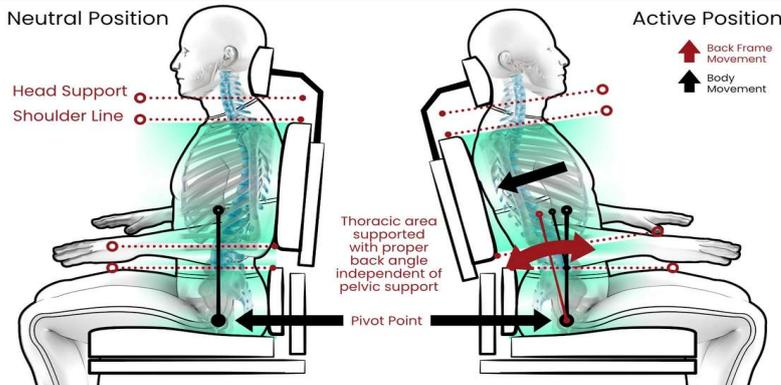
The segmented back support system provides stationary pelvic support and a moving thoracic segment. The system also incorporates an anatomical pivot point, contributing to improved stability. Postural changes can help support functions such as respiration, digestion, peer engagement, fatigue management, and performing routine movements, to name a few. All secondary positioning supports attached to the thoracic segment move in unison with the body, reducing the frequency of repositioning events.
